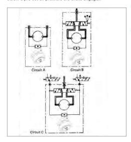
CIRCUIT (A): installation without control valve. The shuttle valve allows brake operation for dual rotation.
