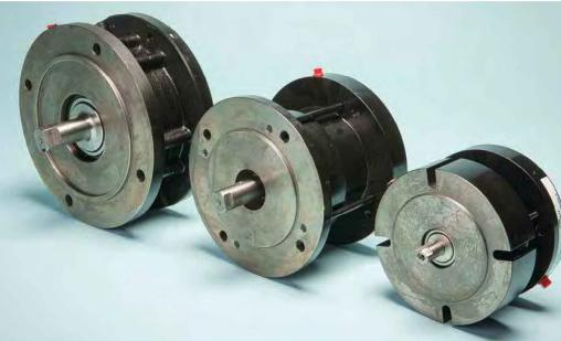
GLOBE BN brakes are fail-safe brakes (spring engaged, air released). They can be used as a static brake and under certain conditions in dynamic applications. The brake module bolts directly onto the motor mounting face with an IEC or NEMA connection flange. The brakes are certified according to the European Explosive Directive ATEX II cat. 2 G&D T3 (in static applications only).
